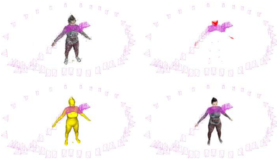
Figure 2.4: Results from various steps of the pipeline. First row: SfM pointcloud and cameras and 3D landmarks; Second row: reconstructed mesh and the fitted template mesh
