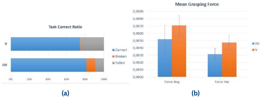
Figure 7.4: Results of the pick-and-place task: (a) Correct rate measured in the pick-and-place tasks. (b) The mean values of the virtual grasping force. With the haptic feedback enabled (HV) interaction forces are reduced.
