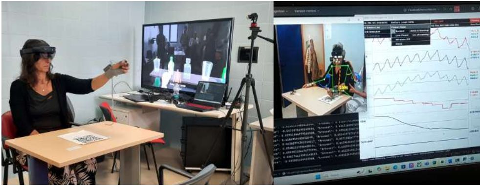
Figure 20.1: (Left) the clinical setup for the Use Case 1: Upper Limb Rehabilitation, including the XR visualization of the virtual exercise (streamed to the external monitor), the haptic glove for interaction and postural tactile hints, the Emotibit armband, and the external camera for upper limb tracking and biometric signals recording. (Right) screenshot of the real-time streaming of the measured data, showing upper limb tracking and physiological signals.
