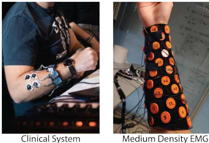
Figure 11.1: (Left) Picture of the gold standard EMG system used (Noraxon desk DTS). (Right) Picture of the Medium-Density EMG system. It consists of 64 monopolar electrodes placed around the forearm of the user.
